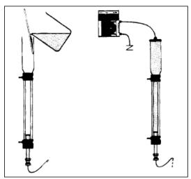
Fig. 1. Packaging the column with GFM.
